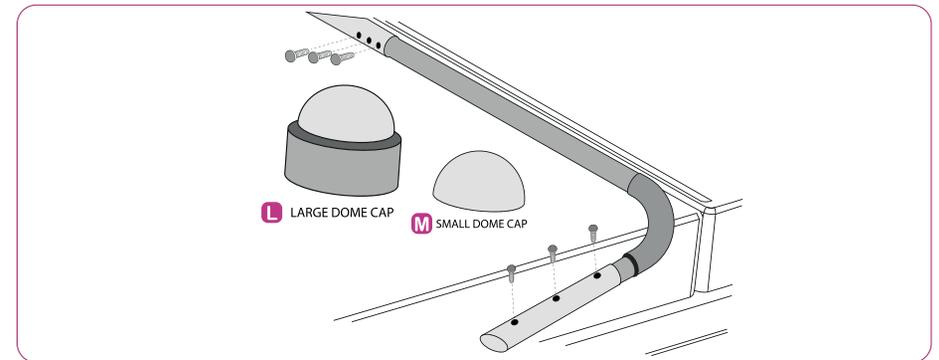
8. Press the decorative Large Black Dome Caps (L) over the heads of the 3/8" x 3" Hex Cap Bolts (L). Then press the decorative Small Black Dome Caps (M) over the heads of all exposed #10 screws (J and K). Note: A small amount of Glue/Epoxy will help secure screw/bolt domes.
