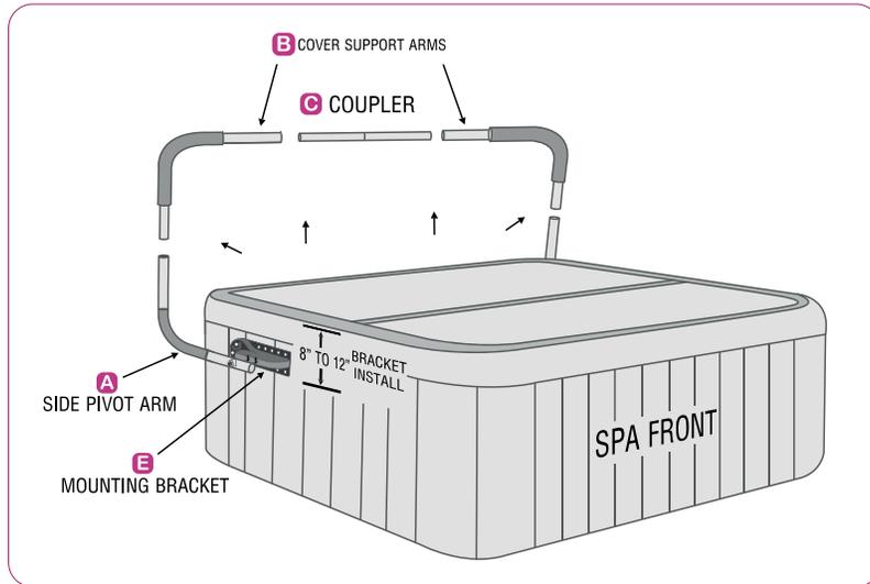
2. Connect the Pivot Arm (A) and two Bushings (D) to the Mounting Brackets (E), using one 3/8" x 3" Hex Cap Bolt (F), two 3/8" Flat Washers (H), and one 3/8" Nylon Locknut (G). REPEAT
